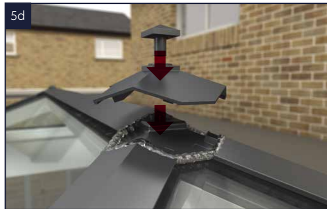
5d Fit the ridge end caps ensuring they are firmly in place.
