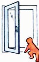
Where small children or mentally handicapped persons have access to the window, the sash is to be safeguarded against turning, for example with a child-safety lock (inhibits turn mode, permits tilt-mode) or key-lockable handle.
