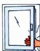
**Caution!** A slamming sash can lead to injuries. While closing, do not grasp between the sash and frame.
