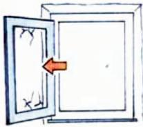
Do not allow the sash to hit or press up against the window reveal.
